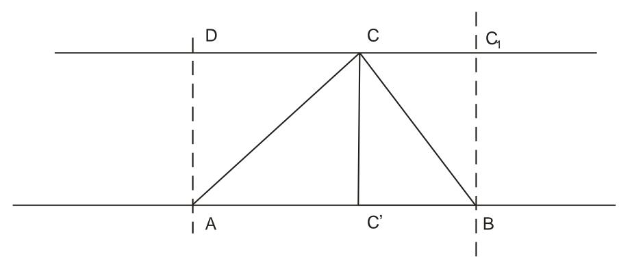
That is, the surface of a triangle is equal to the ½ of the product of the side and corresponding height or is equal to ½ of the product of two legs of a right triangle where one leg is equal to a given side and the other above mentioned height (see picture)
