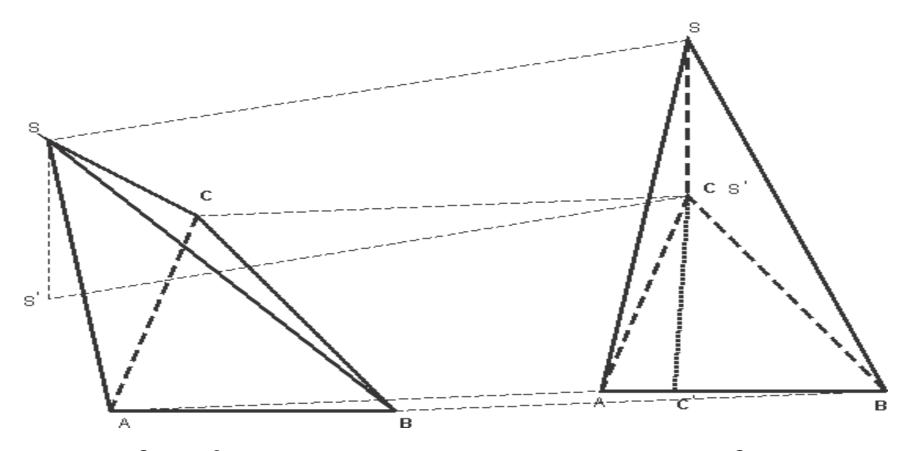
If we bring point S over some vertex of a triangle, for example. C as against its normal projection on the plane of the triangle (ΔABC) and at the same point S does not change the distance from the plane of the triangle, we can see that the distance
